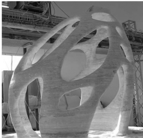
Figure 5. The Radiolaria: Example of full-scale build using the d-shape process
